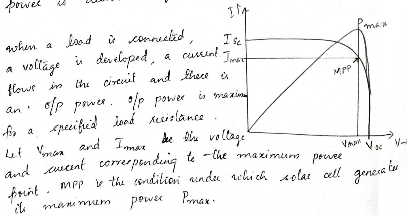
When a load is connected, a voltage is developed, a current flows in the circuit and there is an o/p power. o/p power is maximum for a specified load resistance.
