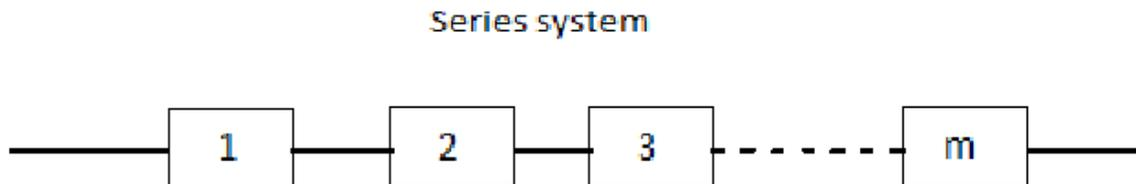
This is the simplest reliability configuration encountered. A series system is shown below. All the components must function successfully for system success. In other words, if any system component fails, the series system fails.
