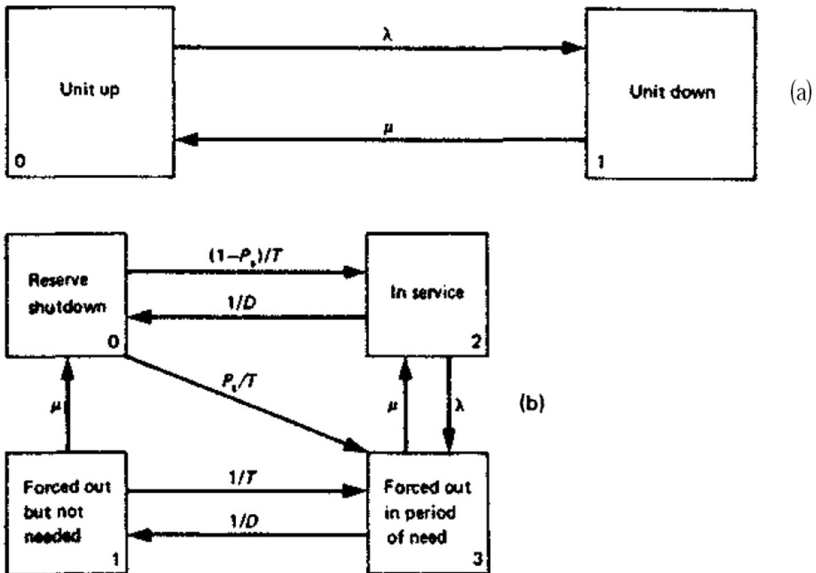
**Fig. 2.3** (a) Two-state model for a base load unit
