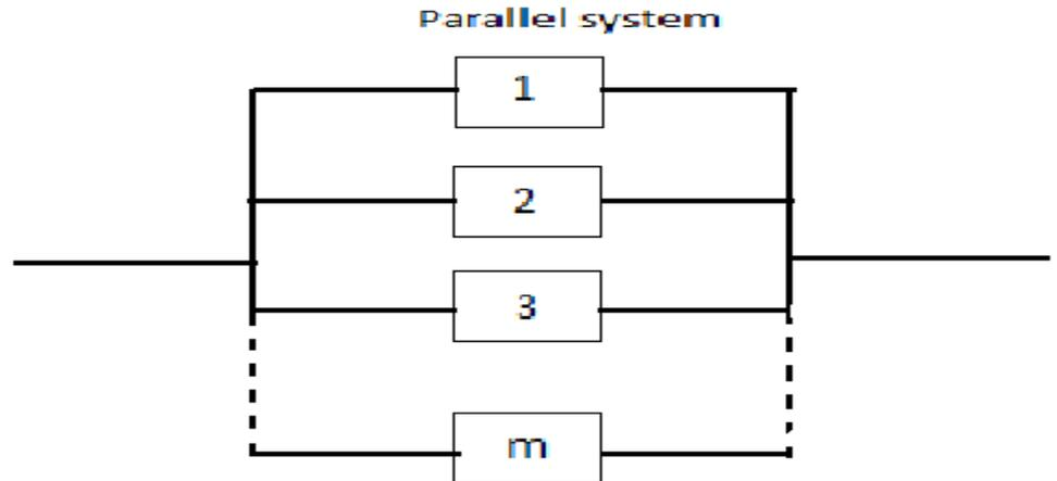
This is a well known configuration used to improve system reliability. All the units of the network are assumed to be active. At least one parallel unit of the network is required for system success. In other words, the system will be successful if at least one network unit is operating successfully. The failure probability of the network shown above is given by
