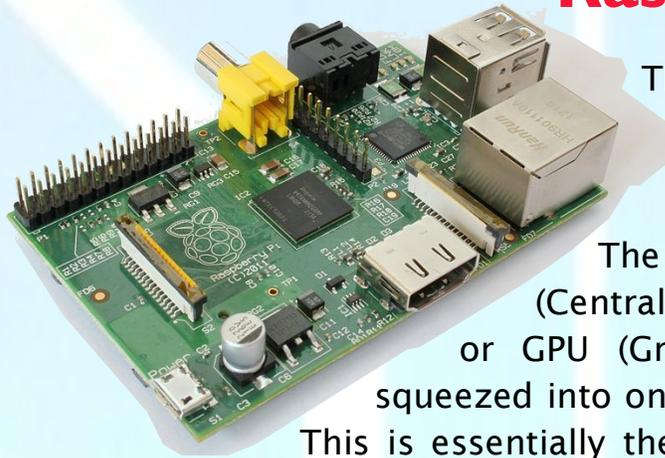
The Raspberry Pi is a credit-card-sized single-board computer developed in the UK by the Raspberry Pi Foundation .
